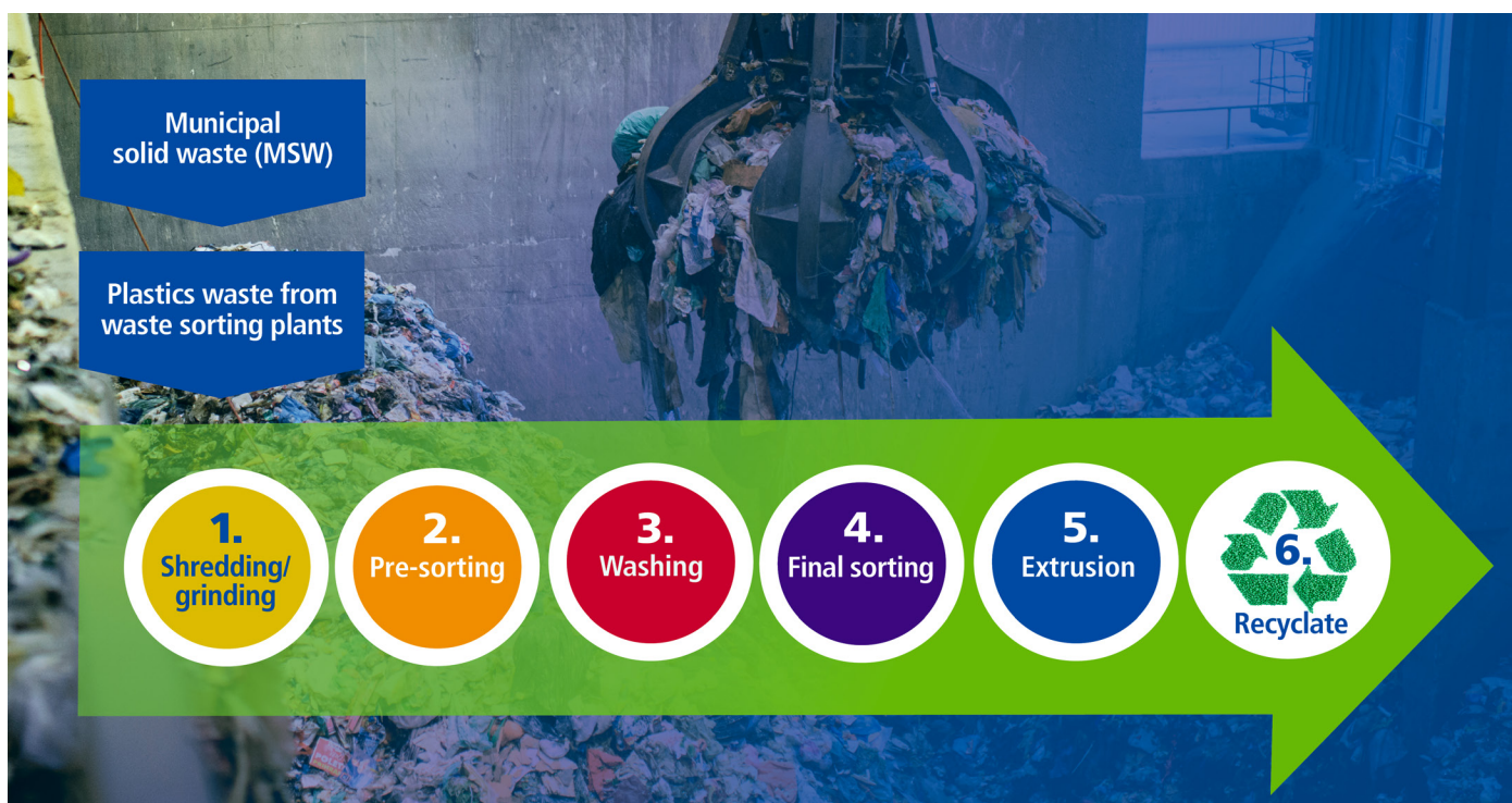
Figure 5. Typical Mechanical Recycling Process.
